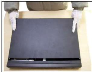
②disassemble the cover
