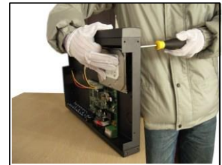
③fix the screw of hard disk
