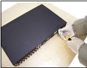
①disassemble the screw
