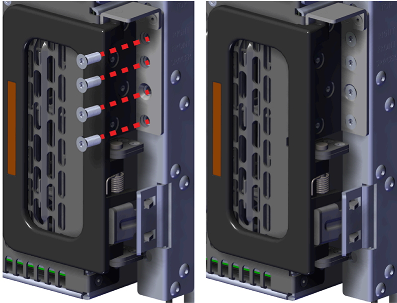
Figure 211: Shipping Bracket Screw Locations (CMA Lite)
