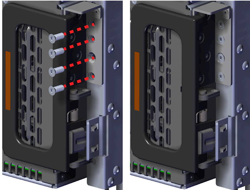
Figure 112: Shipping Bracket Screw Locations (CMA Lite)
