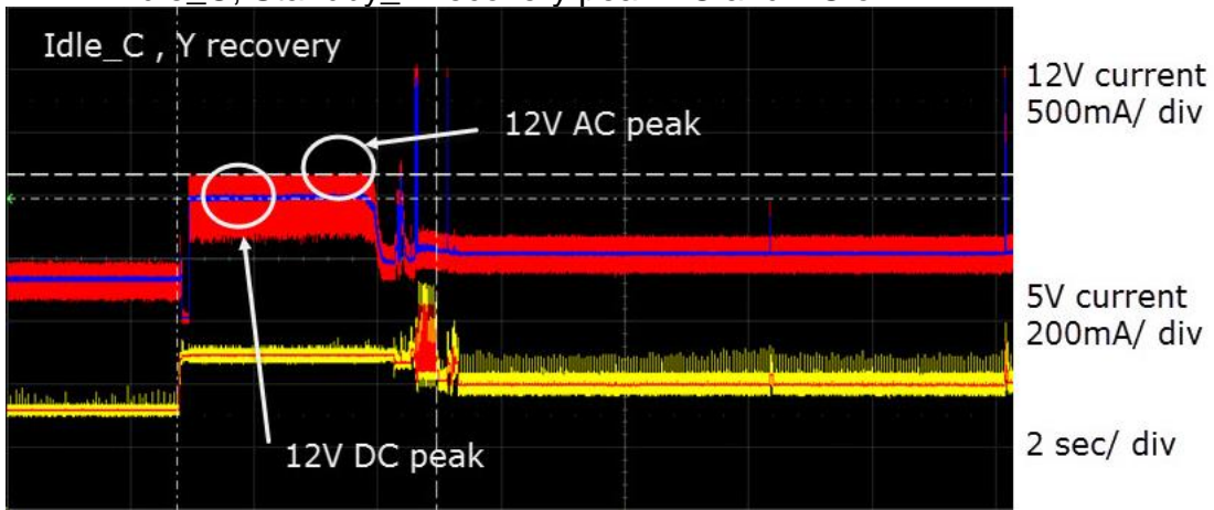
Figure 7 Idle_C Standby_Y recovery current waveform
